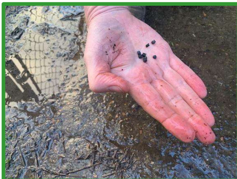
Figure 8 Bio-beads found outside of the entrance to Beckley WTW, April 2021.
