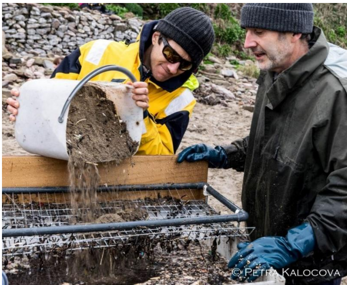
Using the machine to separate microplastics, including Bio-Beads, from the sand, March 2017
