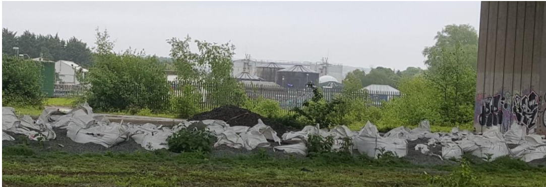
Bio-Beads spilling out of open dumpy sacks in the SWW storage area near the Plympton plant.
